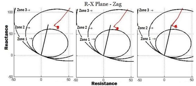
Fig. 5. R-X diagram for the  $Z_{ag}$  unit for the cases without transposition, with ideal transposition, and with actual transposition, respectively.
