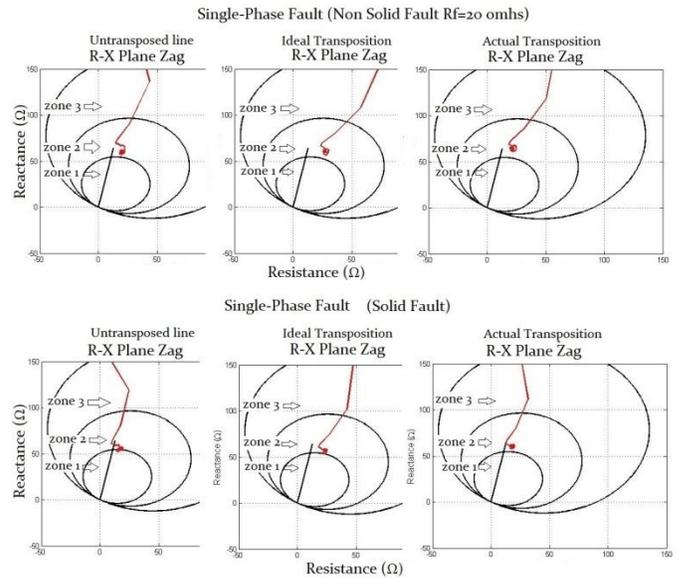
Fig. 19. Influence of considering a non-solid single-phase fault through a 20  $\Omega$  fault resistance when compared to a solid single-phase fault.
