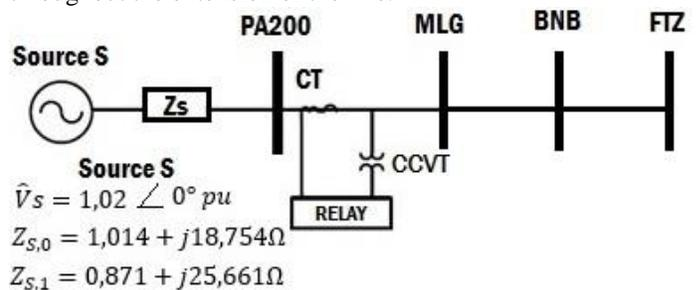
Fig. 2. Electric network implemented.
