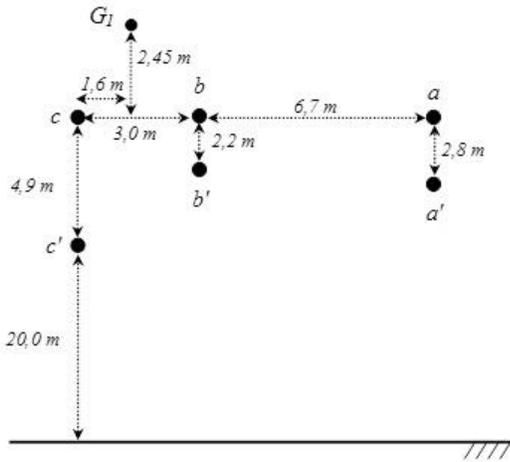
Fig. 3. Conductors geometry
