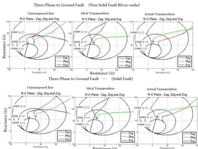
Fig. 21. Influence of considering a non-solid three-phase through a  $20 \Omega$  fault resistance when compared to a solid three-phase fault.
