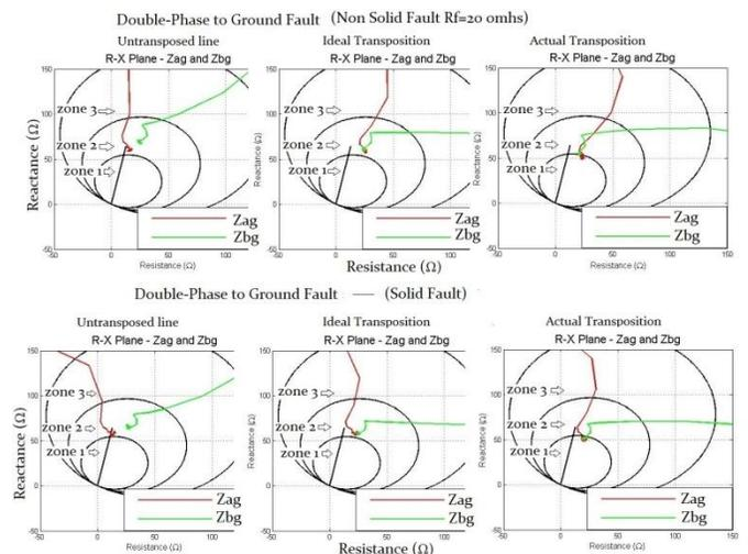
Fig. 20. Influence of considering a non-solid double-phase to ground fault through a 20  $\Omega$  fault resistance when compared to a solid double-phase to ground fault.
