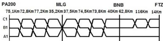
Fig. 4. Actual transposition scheme for the transmission line between Paulo Afonso and Fortaleza.
