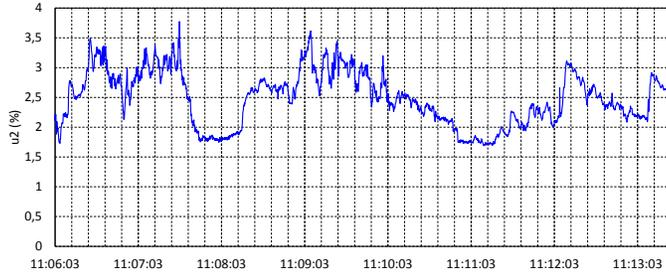
Fig. 22. Voltage unbalance on 110 kV side
