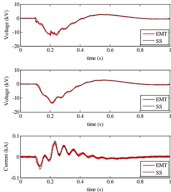
Fig. 3. Changes in (a) Rectifier side DC voltage, (b) Inverter side DC voltage, and (c) DC current for a 0.03 pu, 100 ms pulse applied to the DC voltage reference
