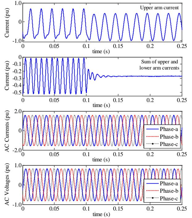
Fig. 8. Simulation results of the circulation current suppression (a) phase-a upper arm current, (b) sum of phase-a arm currents, (c) terminal AC voltages, and (d) AC line currents
