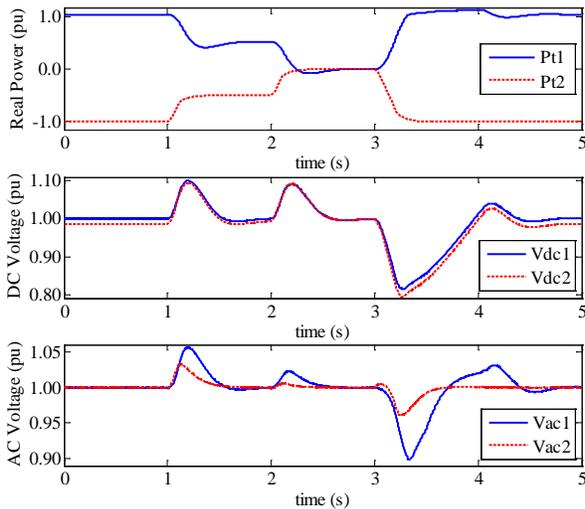
Fig. 5. Simulation results for power order change (a) terminal real powers, (b) DC voltages, and (c) terminal AC voltages
