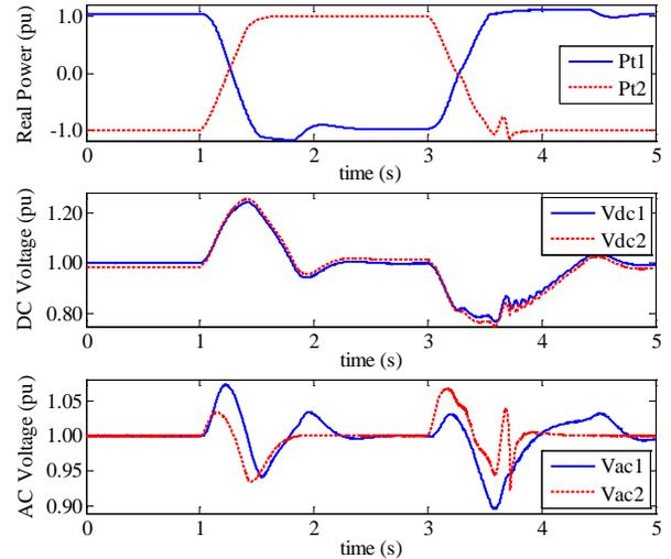
Fig. 6. Simulation results of the power reversal study (a) terminal real powers, (b) DC voltages, and (c) terminal AC voltages
