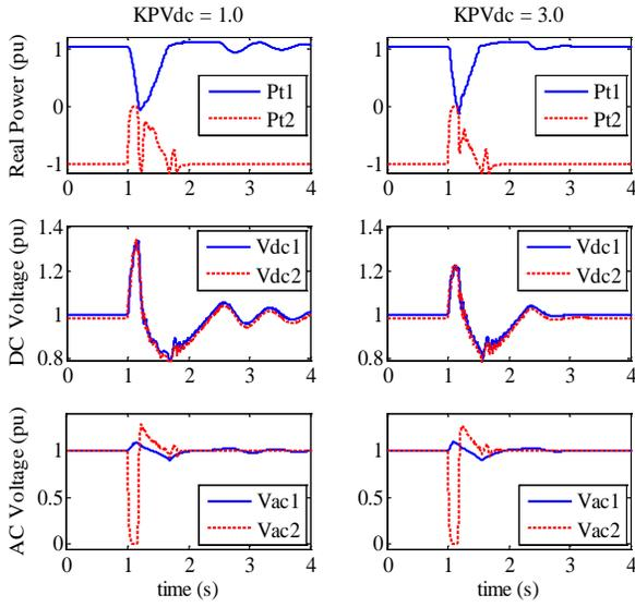
Fig. 10. Simulation results for three phase fault at MMC-2 network terminal (a) terminal real powers, (b) DC voltages and, (c) terminal AC voltages
