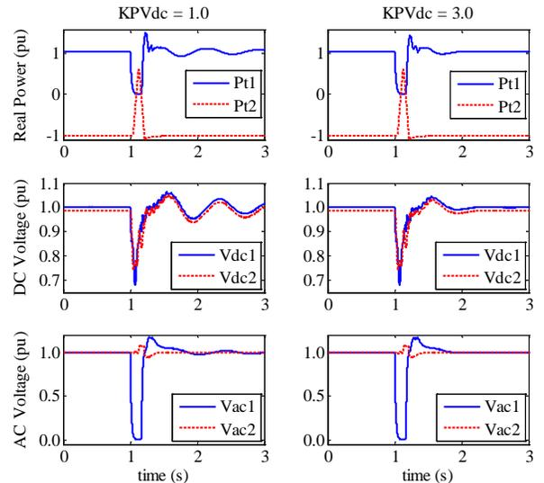
Fig. 9. Simulation results for a three phase fault at MMC-1 network terminal (a) terminal real powers, (b) DC voltages and, (c) terminal AC voltages
