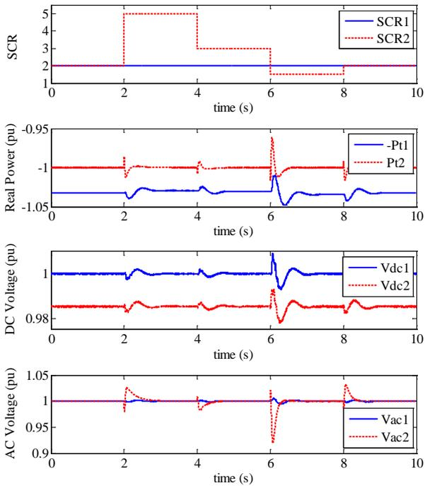
Fig. 7. Simulation results for change in SCR-2 (a) SCR values, (b) terminal real powers, (c) DC voltages, and (d) terminal AC voltages
