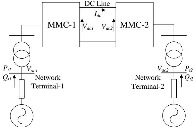
Fig. 1. A point-to-point MMC-VSC system with AC network connections
