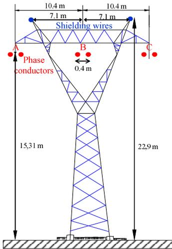
Fig. 2. Conductor arrangement at tower and average heights above the ground
