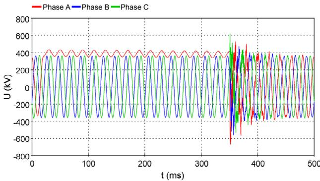
Fig. 16. Voltages at the end of transmission line in case of uncontrolled reclosing in phase A from the beginning of the line
