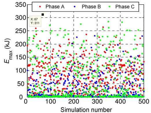
Fig. 7. Energy stress of station surge arresters at the end of transmission line (uncontrolled energization)
