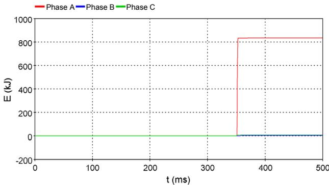
Fig. 17. Energy stress of station surge arresters at the end of transmission line
