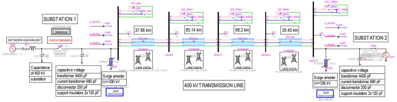
Fig. 1. Model of 400 kV transmission line and substations in EMTP-RV
