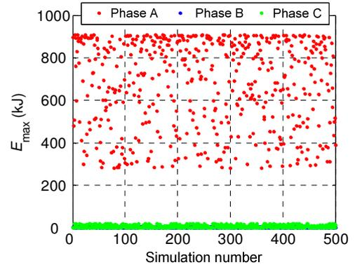
Fig. 20. Energy stress of station surge arresters at the end of transmission line (uncontrolled reclosing)
