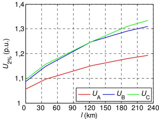
Fig. 10.  $U_{2\%}$  phase-to-ground SOV profiles along the transmission line length (controlled energization)
