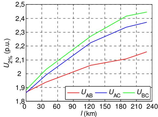
Fig. 11.  $U_{2\%}$  phase-to-phase SOV profiles along the transmission line length (controlled energization)
