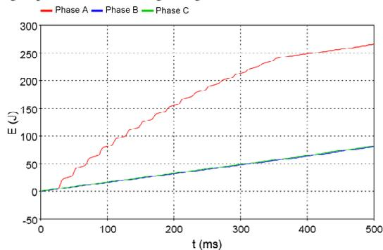
Fig. 22. Energy stress of station surge arresters at the end of transmission line
