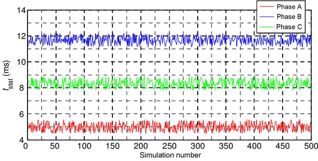
Fig. 9. Closing time of a circuit breaker contacts for 500 switching operations
