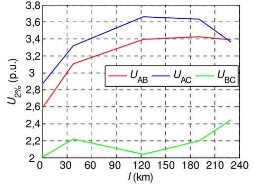
Fig. 19.  $U_{2\%}$  phase-to-phase SOV profiles along the transmission line length (uncontrolled reclosing)
