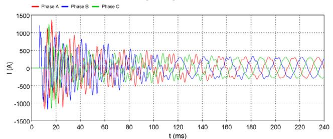
Fig. 8. Currents caused by uncontrolled energization of transmission line ( $I_{\max A}=1365.9$  A,  $I_{\max B}=1213.8$  A,  $I_{\max C}=1263.5$  A)
