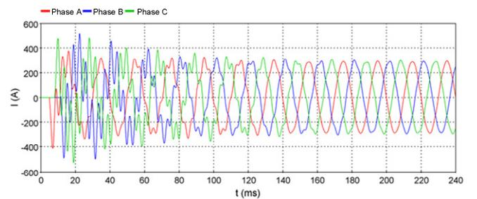
Fig. 15. Currents caused by controlled energization of transmission line ( $I_{\max A}=-415.5$  A,  $I_{\max B}=-513.7$  A,  $I_{\max C}=-528.2$  A)
