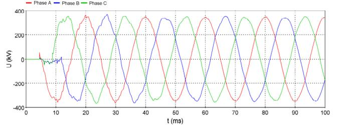
Fig. 12. SOVs at the beginning of the line (controlled energization)
