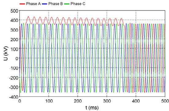
Fig. 21. Voltages at the end of transmission line in case of controlled reclosing in phase A from the beginning of the line
