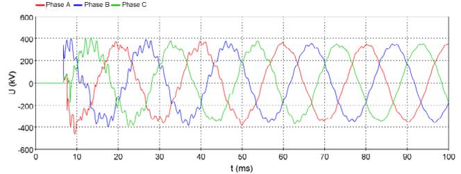
Fig. 5. SOVs at the beginning of the line (uncontrolled energization)
