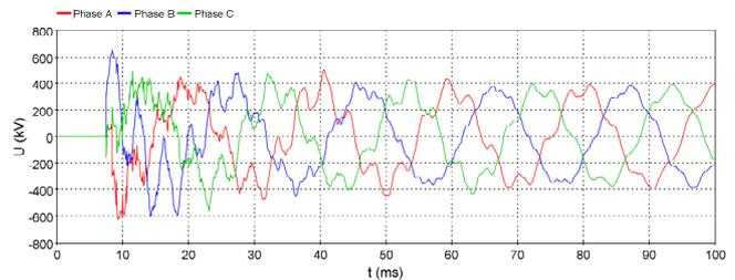
Fig. 6. SOVs at the end of the line (uncontrolled energization)
