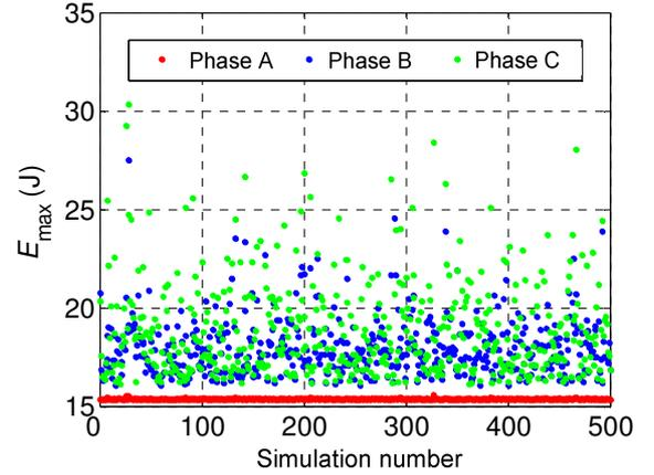
Fig. 14. Energy stress of station surge arresters at the end of transmission line (controlled energization)
