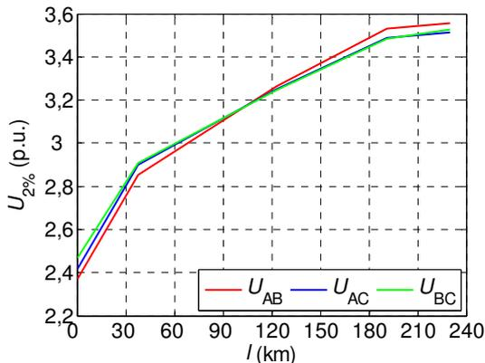
Fig. 4.  $U_{2\%}$  phase-to-phase SOV profiles along the transmission line length (uncontrolled energization)
