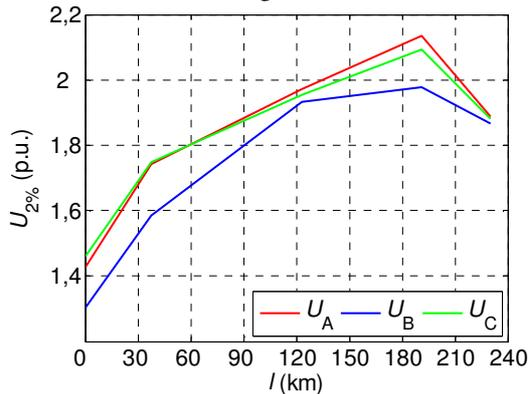
Fig. 3.  $U_{2\%}$  phase-to-ground SOV profiles along the transmission line length (uncontrolled energization)
