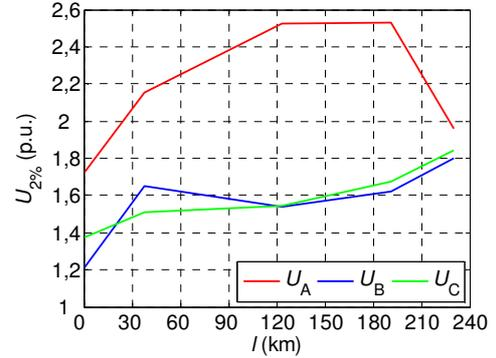
Fig. 18.  $U_{2\%}$  phase-to-ground SOV profiles along the transmission line length (uncontrolled reclosing)
