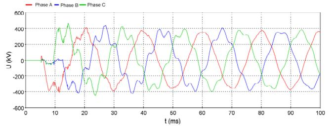
Fig. 13. SOVs at the end of the line (controlled energization)
