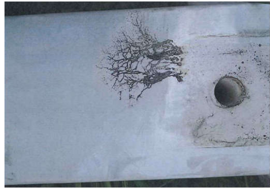
Fig. 8. Surface tracking at top crossarm
