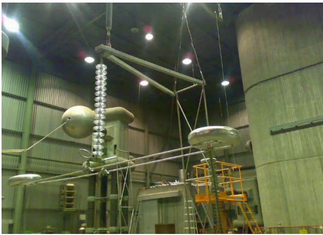
Fig. 2. Test set up for dielectric test on 275kV FRP crossarm
