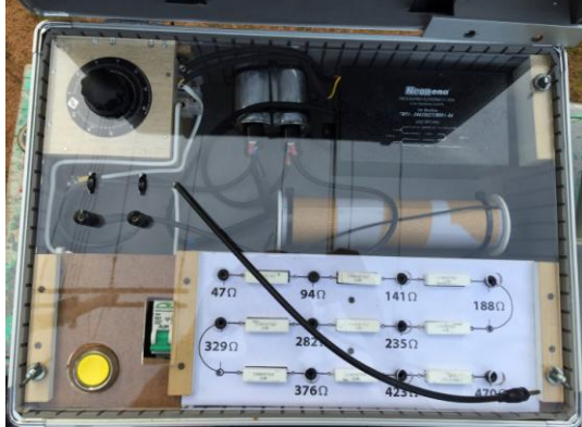
Fig. 1. Voltage impulse generator prototype.
