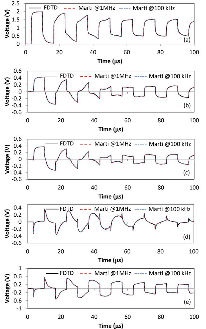
Fig. 4. Voltages at the receiving end of the line for bare phase cables and 1000- $\Omega$ m soil: (a) phase A; (b) phase B; (c) phase C; (d) messenger; (e) neutral. Tested model: Marti's model with complex poles in the fitting of  $Z_c(\omega)$  and  $A(\omega)$ , simulated in Matlab. Reference model: FDTD.
