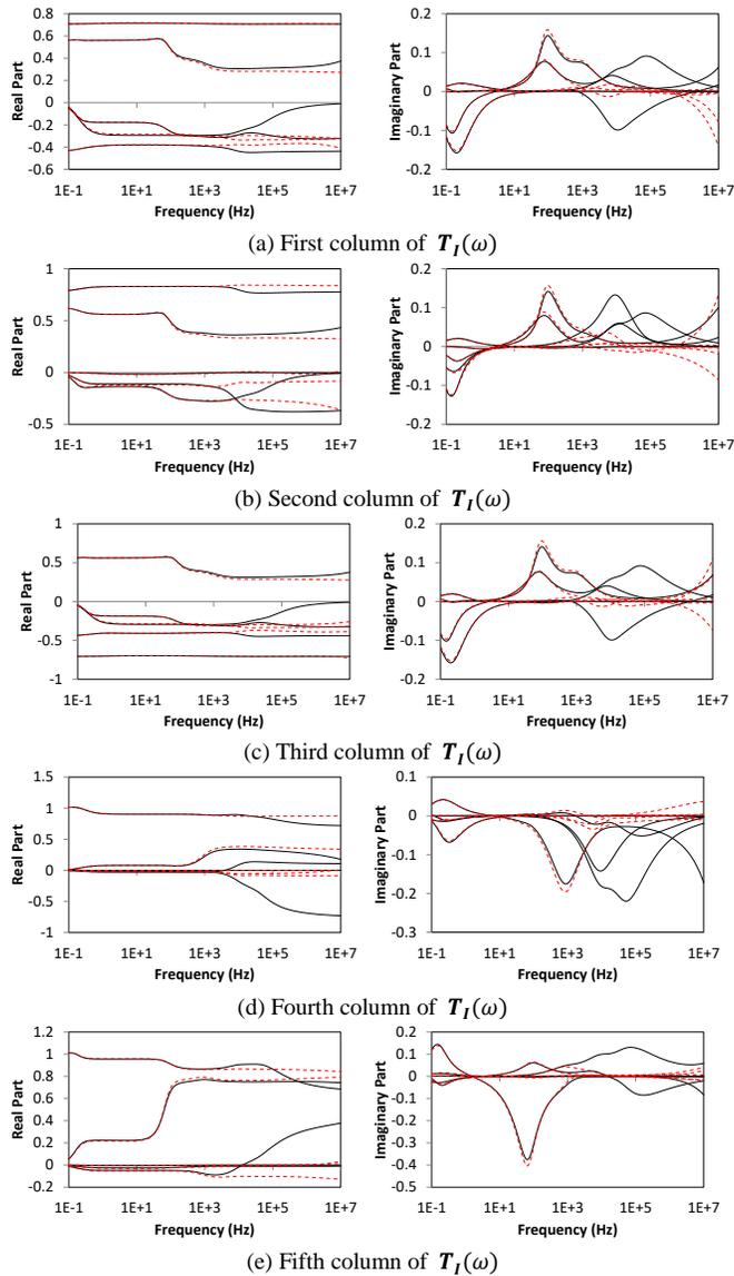
Fig. 3. Elements of the transformation matrix. Solid lines: insulated phase cables; dashed lines: bare phase cables.
