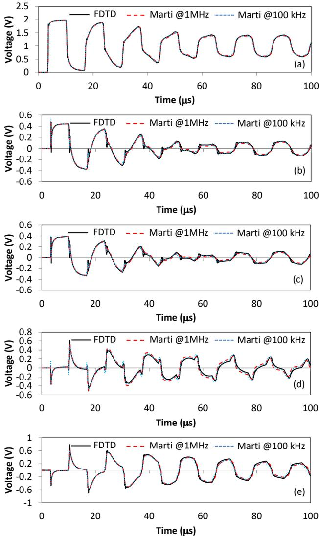
Fig. 5. Voltages at the receiving end of the line for insulated phase cables and 1000-Ωm soil: (a) phase A; (b) phase B; (c) phase C; (d) messenger; (e) neutral. Tested model: Marti's model with complex poles in the fitting of  $Z_c(\omega)$  and  $A(\omega)$ , simulated in Matlab. Reference model: FDTD.
