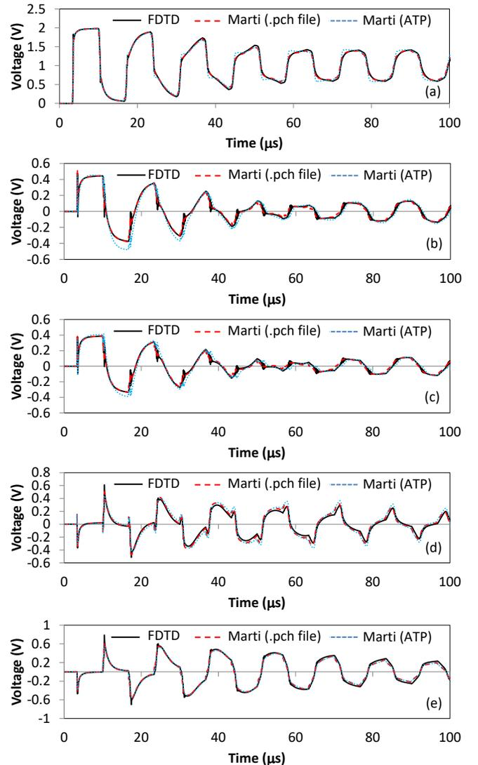
Fig. 6. Voltages at the receiving end of the line calculated for a 1000-Ωm soil assuming insulated phase cables and real poles in the fitting of  $Z_c(\omega)$  and  $A(\omega)$  for simulation with Marti's model in ATP: (a) phase A; (b) phase B; (c) phase C; (d) messenger; (e) neutral.
