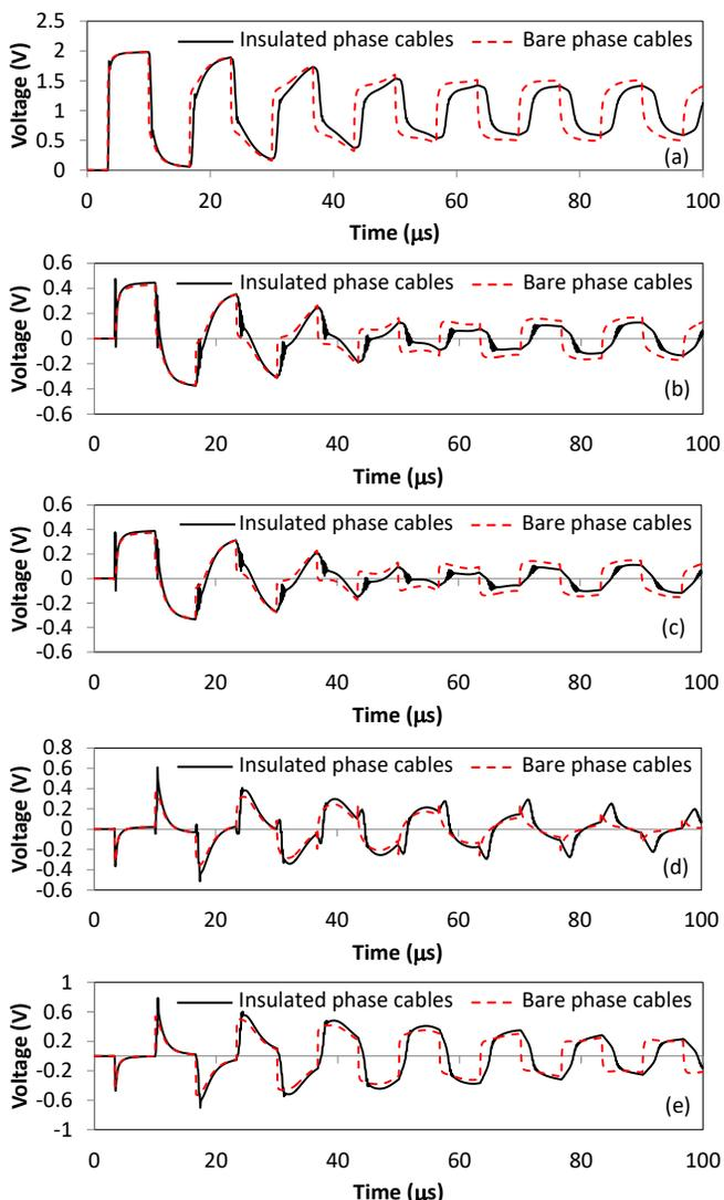
Fig. 2. Voltages at the receiving end of the line calculated for a 1000- $\Omega$ m soil with the FDTD method: (a) phase A; (b) phase B; (c) phase C; (d) messenger; (e) neutral.
