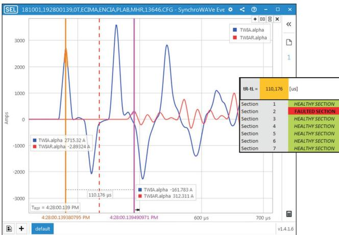
Fig. 7. Obtained results in Case 2: Fault within Section 2 at 80% of  $l_2$ .
