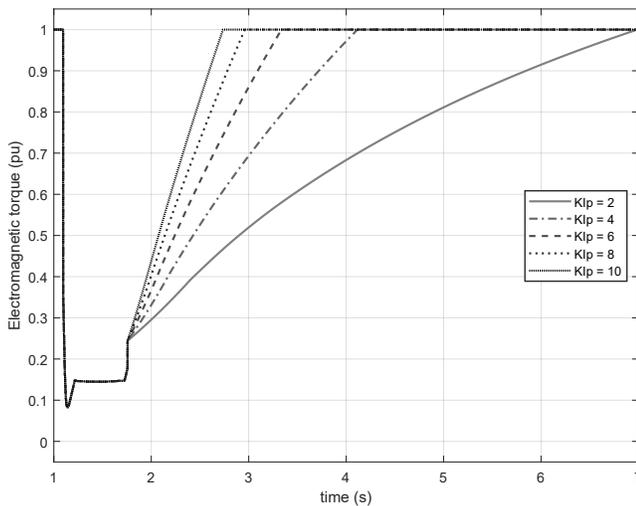
Fig. 9. Effect of varying  $KIp$  in electromagnetic torque.
