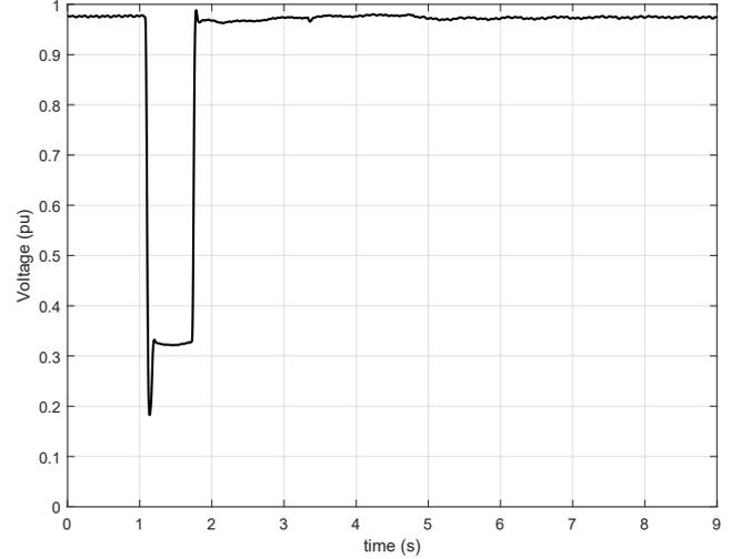
Fig. 4. Three-phase voltage dip voltage profile.
