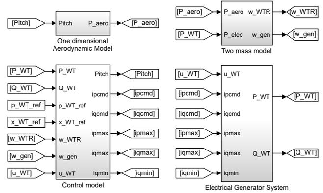
Fig. 1. General structure of a generic Type 3 WT defined by IEC 61400-27-1
