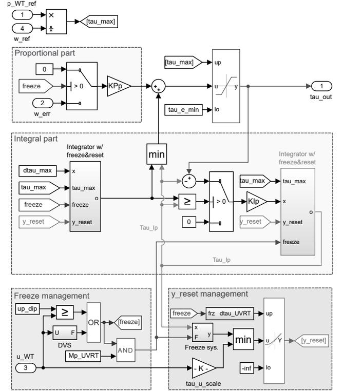
Fig. 3. Electromagnetic torque control system.
