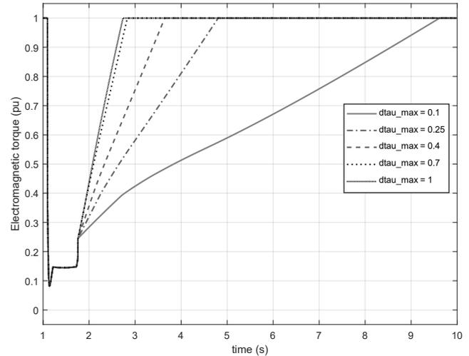
Fig. 8. Effect of varying  $dtau_{max}$  in electromagnetic torque.
