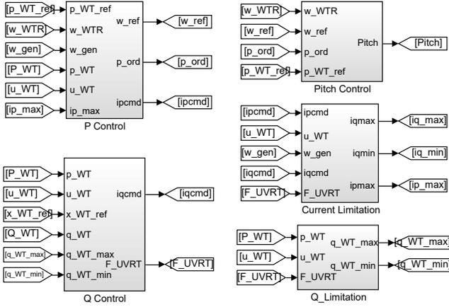
Fig. 2. Control systems included the 'Control model'
