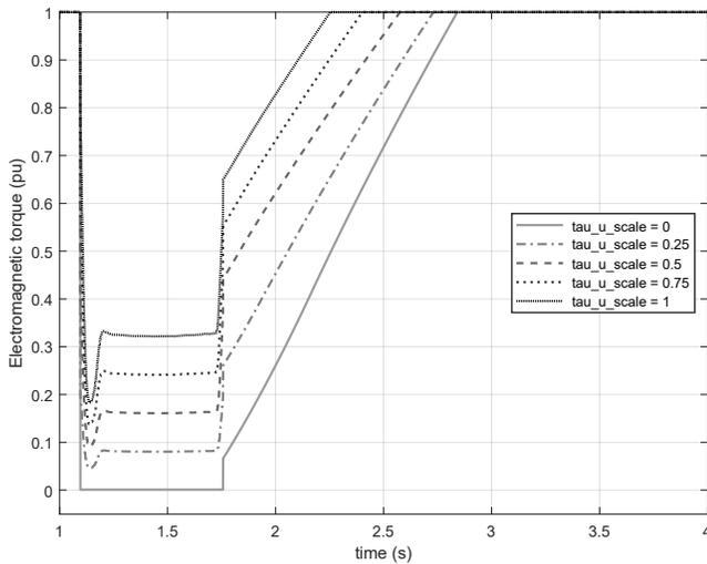
Fig. 5. Effect of varying  $\tau_{u\_scale}$  in electromagnetic torque.
