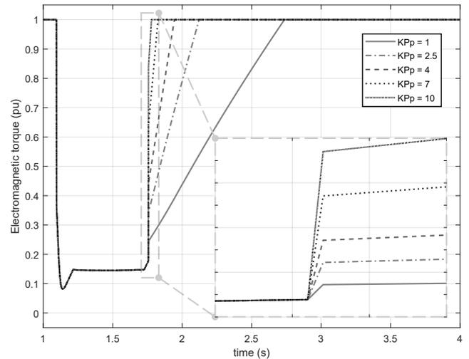
Fig. 7. Effect of varying  $KPp$  in electromagnetic torque.
