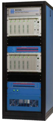
Fig. 1. Real-time simulator for closed-loop simulation from RTDS
