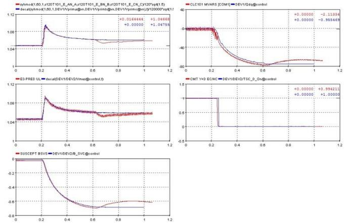
Fig. 2. EMTP-RV SVC101 model behavior (blue) compared to field measurements (red). Left column: direct-sequence voltage (p.u.), measured voltage (p.u.) and SVC101 susceptance (p.u.). Right column: reactive power (Mvar) and TSC state (delta winding). The EMTP-RV model does not represent the current order ramp during the startup sequence, hence the difference at 0.6 s.
