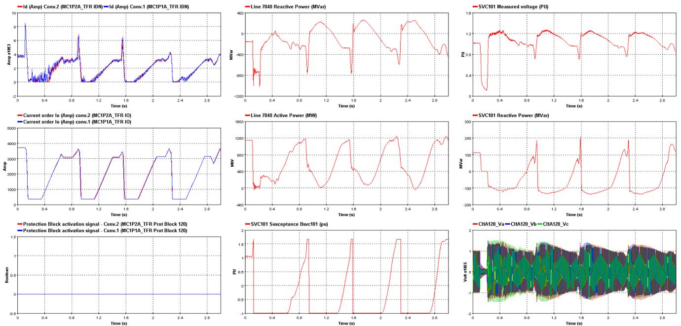
Fig. 7. ABCG fault (14 ms point on wave) at Châteauguay 120 kV bus with SVC101 in service only; 4 Beauharnois units in service (power recovery failed due to bang ramp lock activation). To speed up testing of all cases, the lock itself was deactivated but post-processing of results detects the numerous bang ramps and counts this as a failed power recovery.
