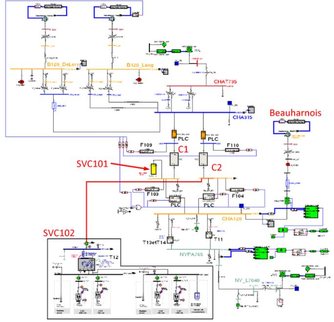
Fig. 4. Hypersim simulation schematic of the Châteauguay-Beauharnois interconnection.
