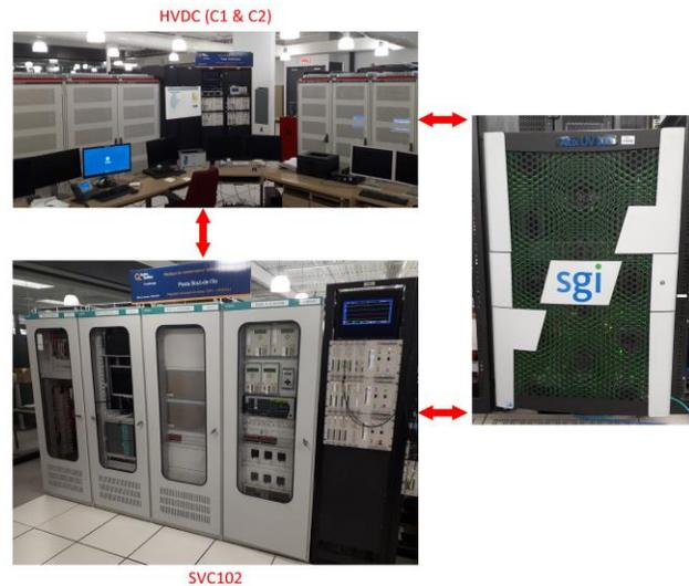
Fig. 5. Hypersim RT HIL setup with SVC and HVDC control system replicas: ABB HVDC and Siemens SVC control replicas and SGI supercomputer for RT simulation.
