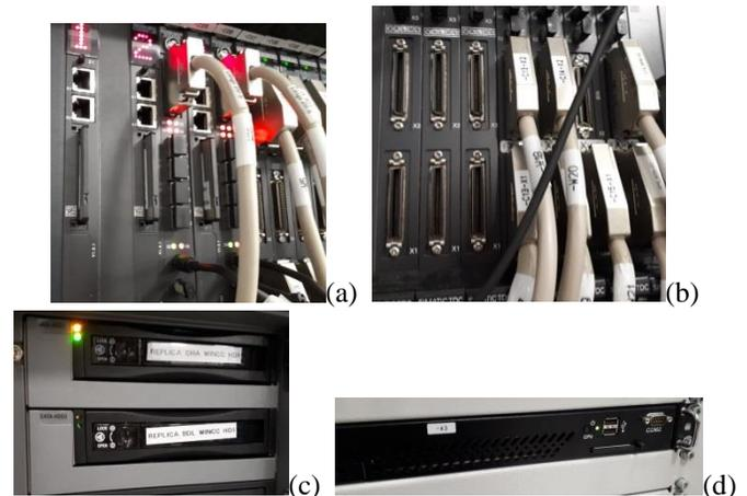
Fig. 3. Toggling between the two configurations involves (a) changing the control software (3 memory cards), (b) rerouting the IOs to the proper IO rack (7 cables), (c) switching the operator workstation hard drive and (d) changing the SCADA memory card.
