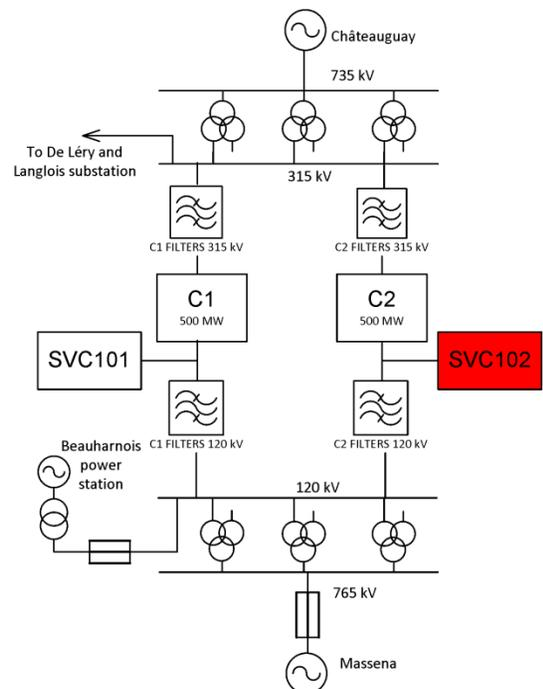
Fig. 1. Schematic of Châteauguay interconnection illustrating both converters (C1 and C2), their 315 and 120 kV filter banks (the icon represents both series and shunt filter banks), Beauharnois power station synchronously connected to NYPA power system and both SVCs: SVC101 with analog control system and SVC102 refurbished with digital control system.
