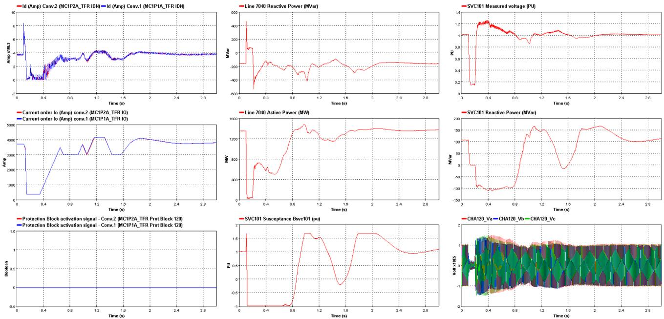
Fig. 6. ABCG fault (0 ms point on wave) at Massena 765 kV bus with SVC101 in service only; 9 Beauharnois units in service (successful power recovery).
