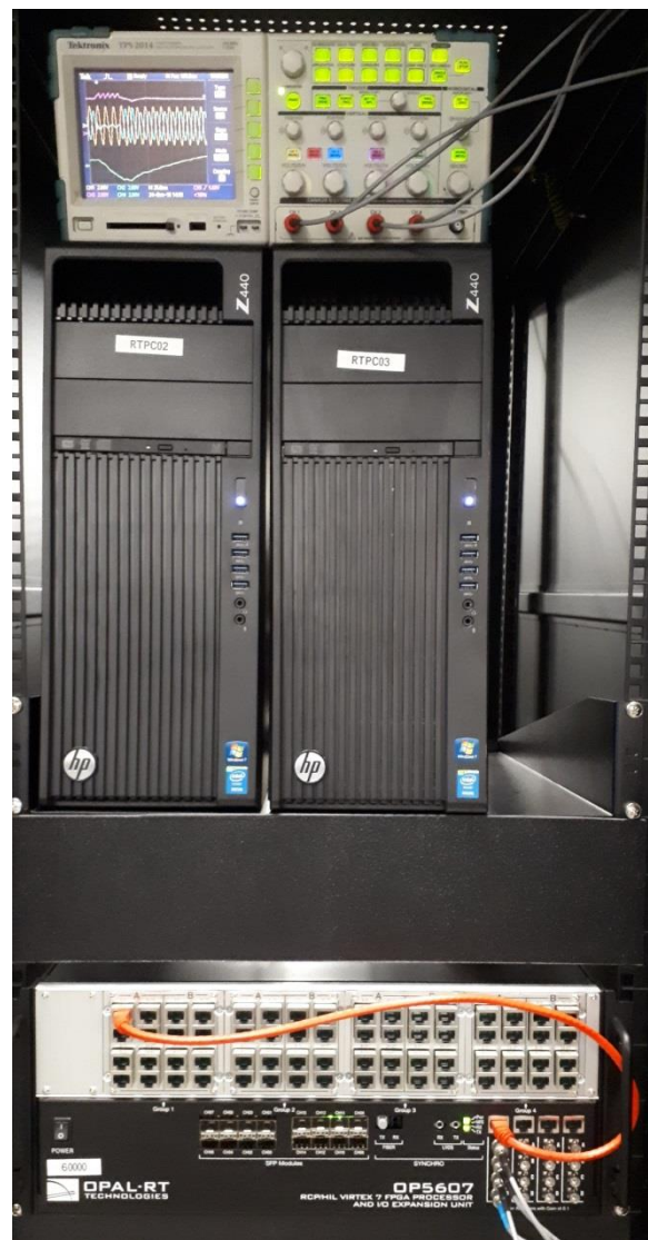
Fig. 4. Simulation setup for the application example: RTPC02 (simulating) and RTPC03 (used for another project) (HP Z440 workstation, Intel Xeon E5-
