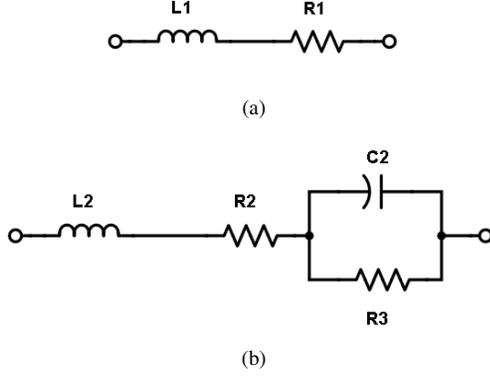
Fig. 7. Series equivalent circuit for (a) real pole, (b) complex pole pair.
