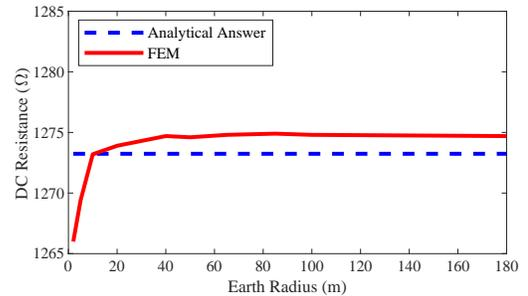
Fig. 3. DC resistance of a PEC hemispherical electrode buried in homogeneous soil as a function of the ground's radius obtained from FEM.
