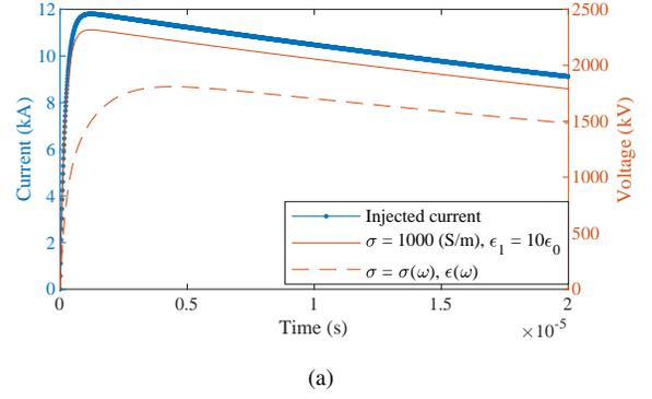
Fig. 8. Simulated GPR of the 5 m vertical grounding electrode under the assumption of constant and frequency-dependent soil parameters.
