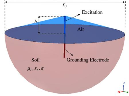
Fig. 1. Proposed FEM model representing the grounding electrode buried in soil (brown hemisphere); The upper-ground part is represented with the blue cone filled with air. The excitation is equivalent to a voltage source of 1V in amplitude (Note that the dimensions are not exact in the figure).
