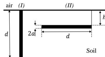
Fig. 4. Vertical (I) and horizontal (II) grounding electrodes buried in homogeneous soil with constant parameters.
