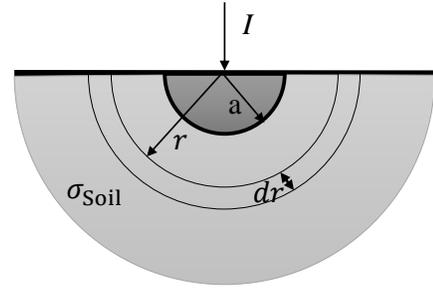
Fig. 2. Current injection in a perfect conducting hemispherical electrode of radius  $r_0$  buried in homogeneous soil with conductivity of  $\sigma_{\text{Soil}}$ ; a differential segment with a radial length of  $dr$  is specified.
