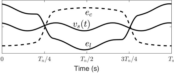
Fig. 2. Simulated wave shapes of the current and voltages saturated oscillations from the circuits shown in Fig. 1.
