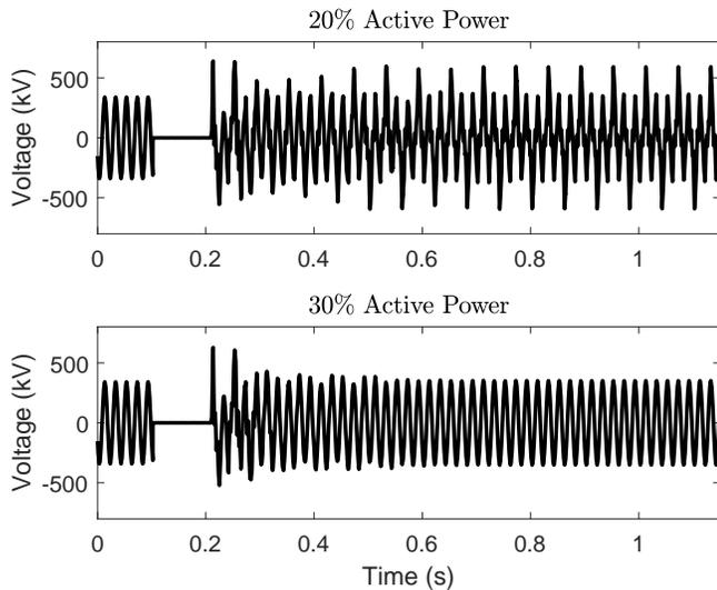
Fig. 12. Voltage waveforms in the transformer station. A three-phase fault was applied on the line between the transformer station and South at  $t = 0.1$  s. The fault was cleared after 100 ms by disconnecting the line.
