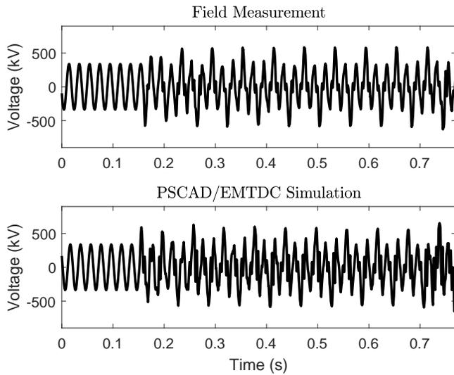
Fig. 5. Phase-to-ground voltage in the transformer station. The upper portion of the figure shows data acquired from field measurements with a sample rate of 12.8 kHz. The bottom portion of the figure shows simulation results.
