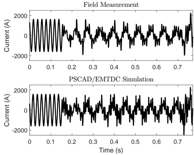
Fig. 7. The series-compensated line's phase current. The upper portion of the figure shows data acquired from field measurements in North with a sample rate of 25.6 kHz. The bottom portion of the figure shows simulation results.
