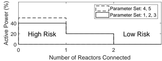
Fig. 13. Ferroresonance risk diagram evaluated based on the transformers' active power and the numbers of reactors connected in the transformer station.
