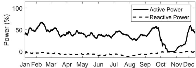
Fig. 14. The load curve of transformer T1 during the year of the disturbance. The load curve is obtained from a power system state estimator.
