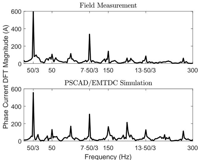
Fig. 10. The DFT magnitude of the series-compensated line's phase current.
