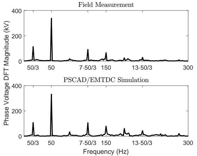
Fig. 8. The DFT magnitude of the phase-to-ground voltage in the transformer station.
