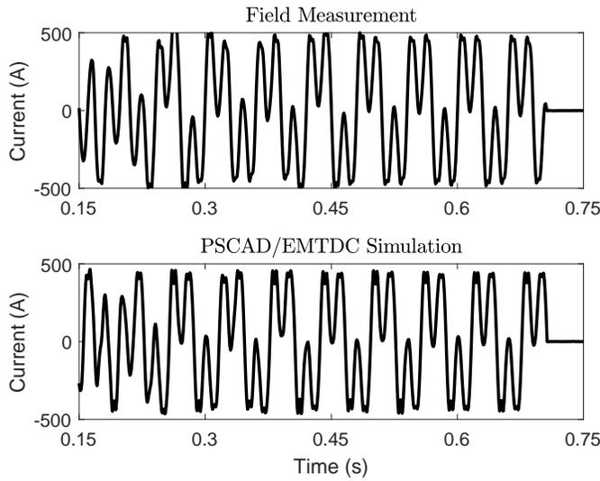
Fig. 6. The reactor's phase current. The upper portion of the figure shows data acquired from field measurements with a sample rate of 1 kHz. The bottom portion of the figure shows simulation results.
