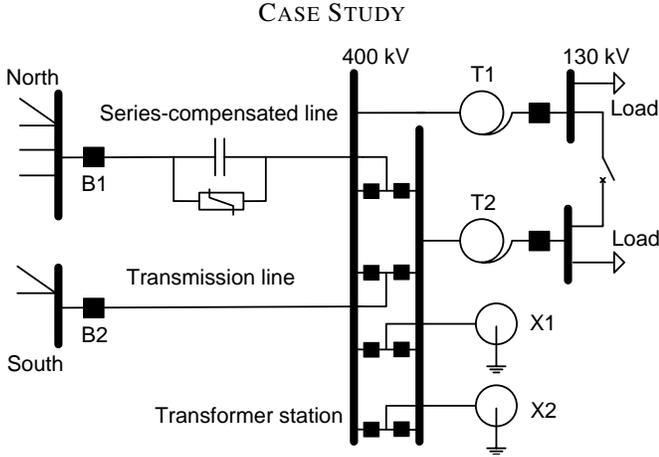
Fig. 3. Critical part of the Swedish power system used in this case study.
