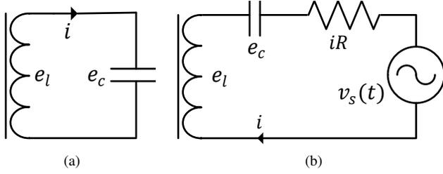
Fig. 1. Simple electric circuits subjected to magnetic saturation. In the oscillatory lossless electric circuit (a), only the natural frequency will be present. In the electric circuit (b), the frequency of the voltage source will be present in addition to the natural frequency.
