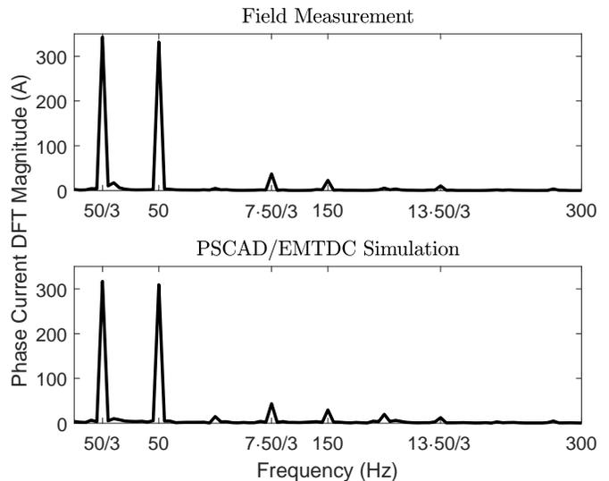
Fig. 9. The DFT magnitude of the reactor's phase current.
