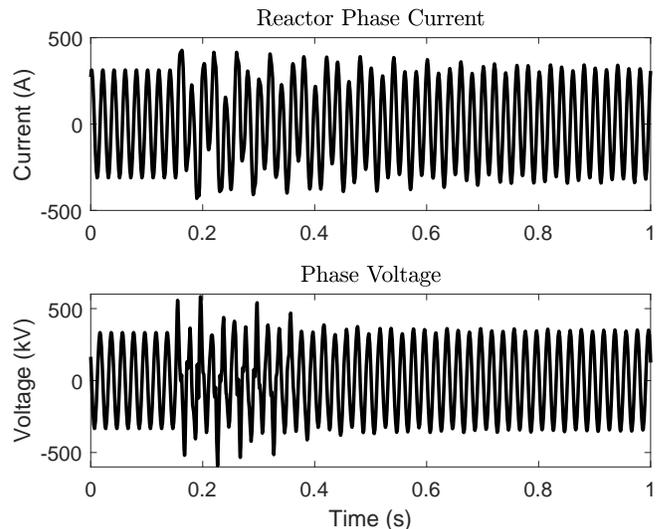
Fig. 11. The reactor's phase current and the phase-to-ground busbar voltage in the transformer station.
