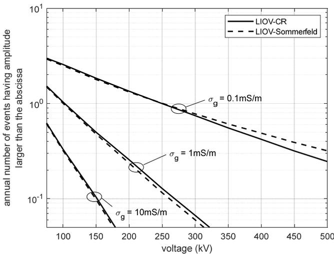
Fig. 9. Lightning performance of the line for different ground conductivities.
