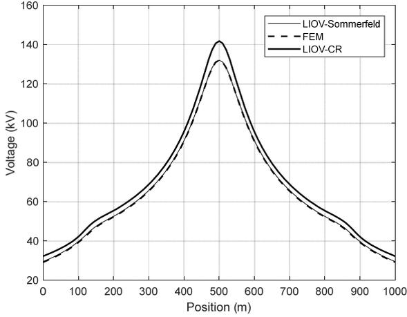
Fig. 5. Overvoltage peak amplitude along the line due to a subsequent stroke.  $\sigma_g = 1$  mS/m.
