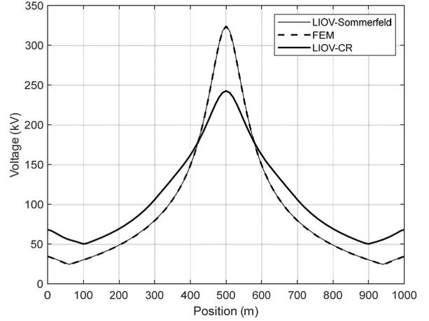
Fig. 8. Overvoltage peak amplitude along the line due to a subsequent stroke.  $\sigma_g = 0.1$  mS/m.
