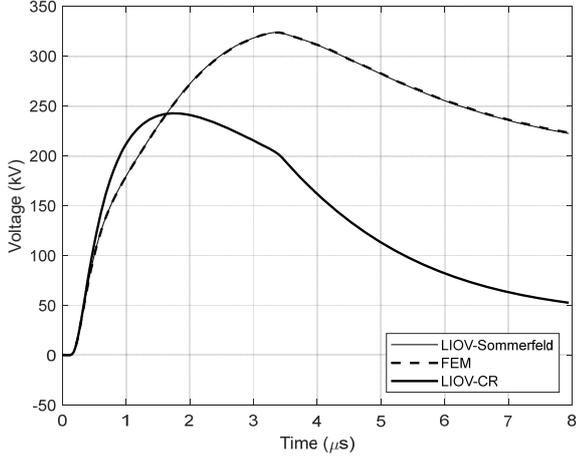
Fig. 6. Overvoltage in the middle of the line due to a subsequent stroke.  $\sigma_g = 0.1$  mS/m.
