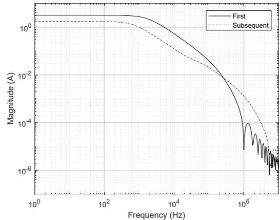
Fig. 1. Magnitude of the Heidler function in frequency domain, approximated with exponentials [19]. Comparison between a typical first and subsequent stroke.
