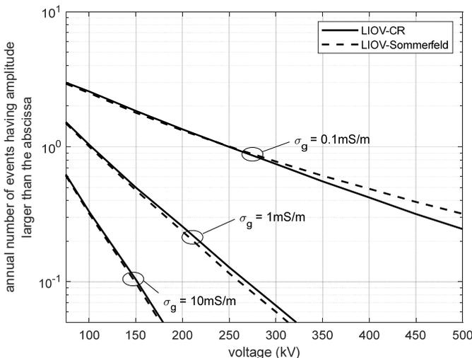
Fig. 9. Lightning performance of the line for different ground conductivities.
