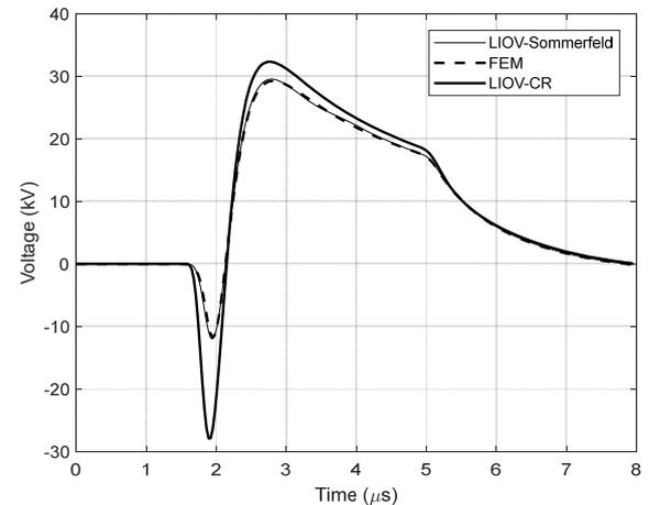
Fig. 4. Overvoltage at line terminations due to a subsequent stroke.  $\sigma_g = 1$  mS/m.
