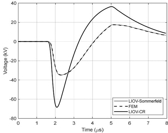
Fig. 7. Overvoltage at line terminations due to a subsequent stroke.  $\sigma_g = 0.1$  mS/m.
