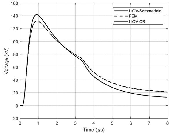
Fig. 3. Overvoltage in the middle of the line due to a subsequent stroke.  $\sigma_g = 1$  mS/m.
