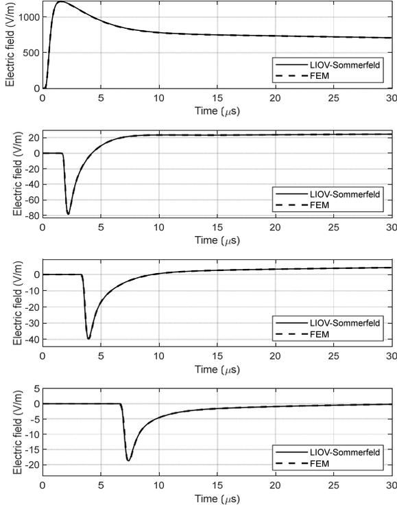
Fig. 2. Radial electric field due to a subsequent stroke calculated at  $r = 51, 502.5, 1001, 2001$  m from the lightning channel.  $\sigma_g = 1$  mS/m.
