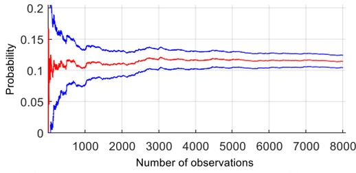
Fig. 2: RMS voltage drop probability of exceeding 5%, depending on the number of simulations, with a confidence interval
