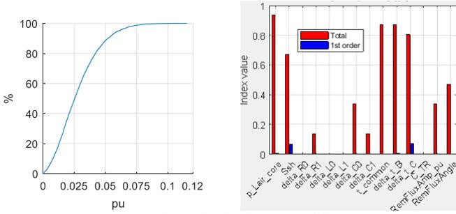
Fig. 3: (a) RMS voltage drop CDF; (b) Sobol sensitivity indices for exceeding the TOV limit
