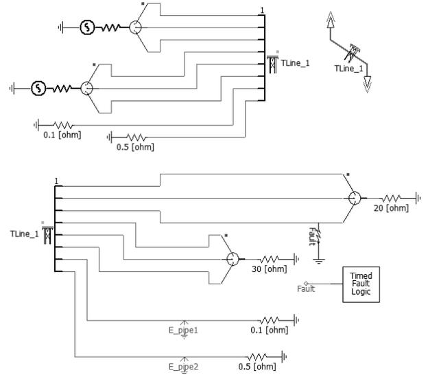
Figure 2. Network configuration for the transient simulation
