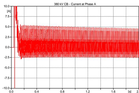
Figure 19. Current of Phase A at the 380 kV circuit breaker (CB<sub>1</sub>)
