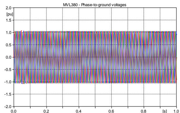
Figure 17. Phase-to-ground voltages at the PCC
