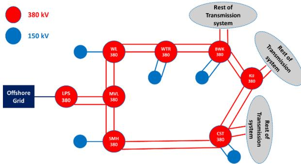
Fig. 3. Simplified representation of the transmission system modelled in EMTP/ATP
