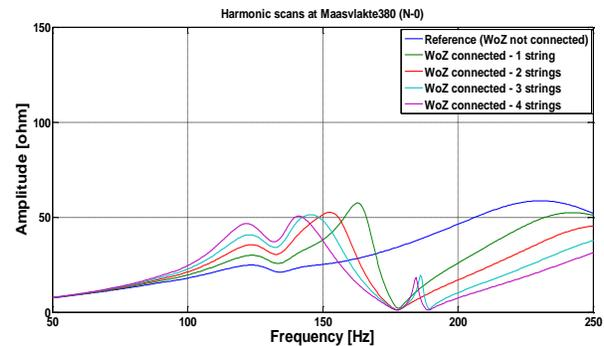
Fig. 4. Harmonic impedance scans at the PCC: N-0 contingency with zero (blue), one (green) up to four (purple) export cables in service
