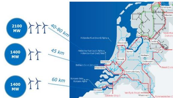
Fig. 1. Connection points of three offshore grids to the 380 kV Dutch transmission system
