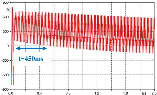
Fig. 9. Current zero-miss – 33 kV reactor not energized
