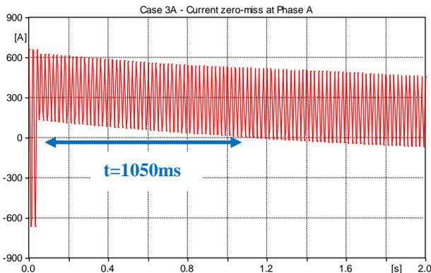
Fig. 10. Current zero-miss – 33 kV reactor already energized
