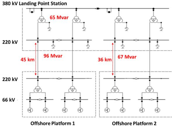
Fig. 2. Single-line diagram of the offshore grid
