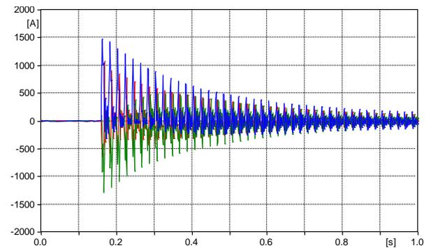
Fig. 14. Non-ideal PoW energization of the offshore transformer – Phase currents at the CB<sub>6</sub> circuit breaker
