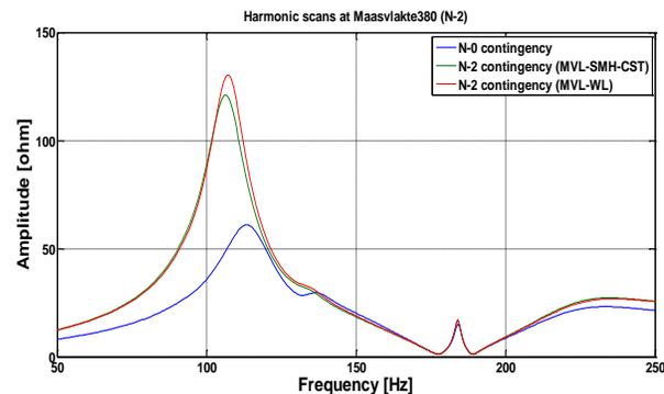
Fig. 5. Harmonic impedance scans at the PCC: N-0 VS N-2 contingencies
