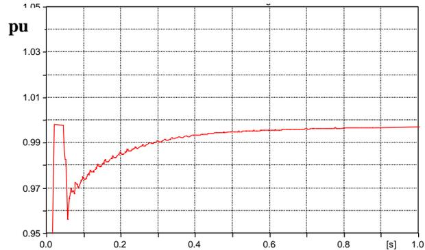
Fig. 12. Non-ideal PoW energization of the offshore transformer – RMS voltage at Phase A of the PCC r
