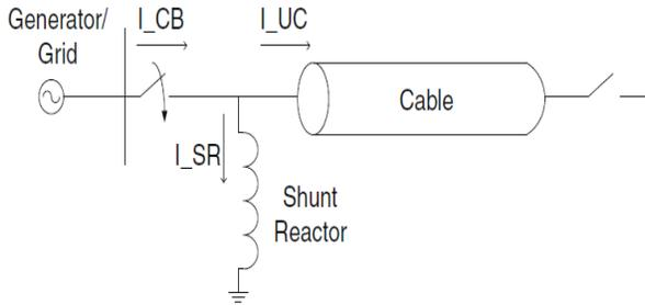
Fig. 6. Simplified representation of the energization of a shunt compensated cable
