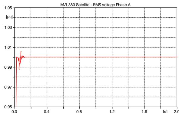
Figure 18. RMS voltage of Phase A at the PCC
