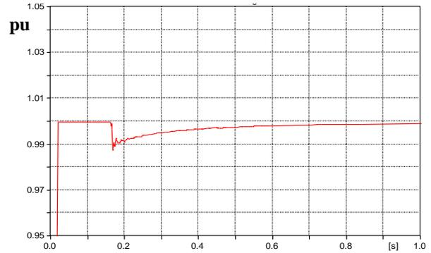
Fig. 11. Ideal PoW energization of the offshore transformer – RMS voltage at Phase A of the PCC
