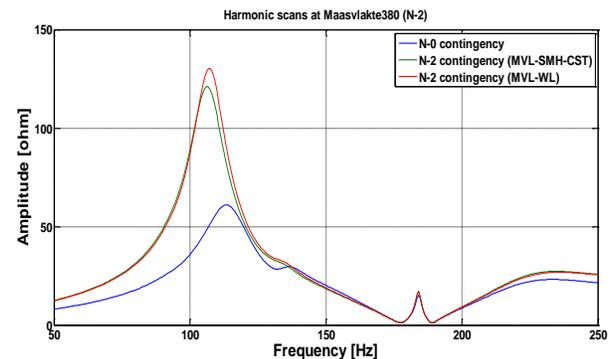
Fig. 5. Harmonic impedance scans at the PCC: N-0 VS N-2 contingencies
