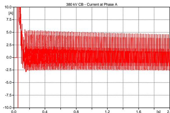
Figure 19. Current of Phase A at the 380 kV circuit breaker ( $CB_1$ )
