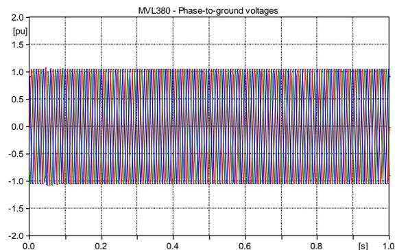
Figure 17. Phase-to-ground voltages at the PCC
