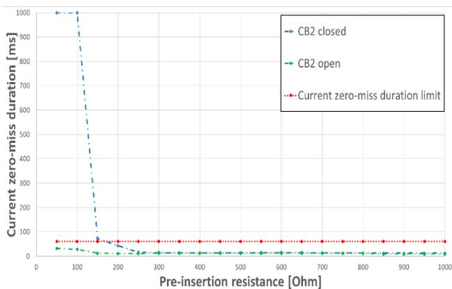
Fig. 16. PIR parametric analysis results
