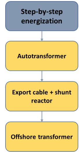
Fig. 8. Step-by-step energization sequence
