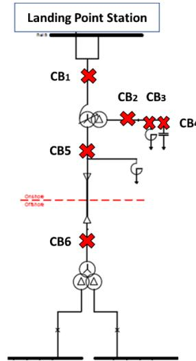
Fig. 7. Circuit breakers in an offshore string
