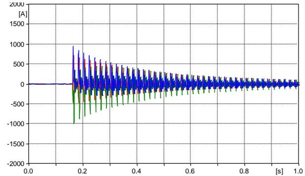
Fig. 13. Ideal PoW energization of the offshore transformer – Phase currents at the CB<sub>6</sub> circuit breaker
