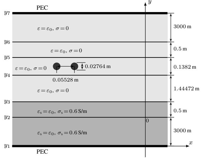
Fig. 1. Depiction of the two-conductor MTL with round conductors situated in two-layer medium consisting of air half-space and lossy half-space and its partitioning into layers. The layered medium is terminated by PEC planes situated at  $y = \pm 3000$ m.
