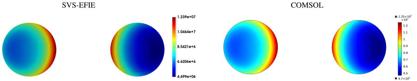
Fig. 2. Volumetric current density in the two-conductor MTL at 60Hz. The centers of conductors are elevated 1.51382m above the soil/air interface. The conductors are driven differentially 1V in the left conductor and 0V in the right conductor. The current distribution computed using SVS-EFIE is shown in the left. The validated result by COMSOL FEM [14] is shown in the right.
