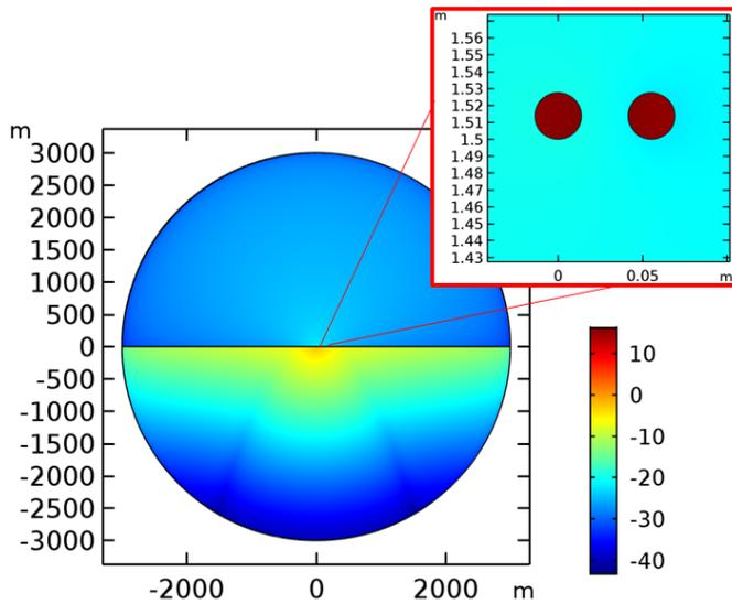
Fig. 4. Model set up and the current density distribution in the conductors and the soil domain computed in COMSOL FEM [14] at 60Hz.
