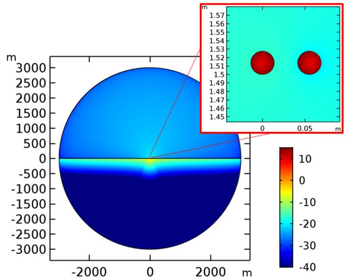
Fig. 5. Model set up and the current density distribution in the conductors and the soil domain computed in COMSOL FEM [14] at 1000Hz.
