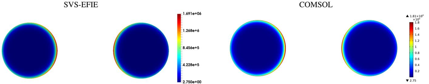
Fig. 3. Volumetric current density in the two-conductor MTL at 5000Hz. The centers of conductors are elevated 1.51382m above the soil/air interface. The conductors are driven differentially 1V in the left conductor and 0V in the right conductor. The current distribution computed using SVS-EFIE is shown in the left. The validated result by COMSOL FEM [14] is shown in the right.
