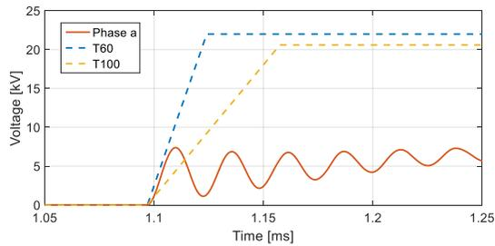
Fig. 5. Worst case for 4.16 kV system (T100 and T60).
