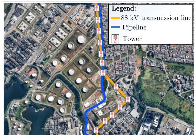
Fig. 5. Top view of the real right-of-way shared between a transmission line and a pipeline.
