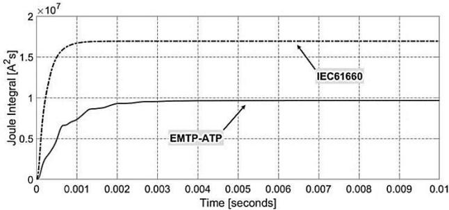
Fig. 8. Joule Integral of the correspondent total short-circuit currents.
