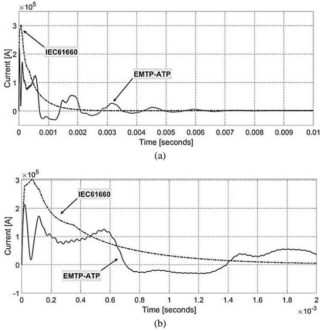
Fig. 7. Total short-circuit current at the fault point of ATP simulation (solid line) and IEC 61660-1 (dashed line). (a) 10 ms time interval. (b) 2 ms time interval.
