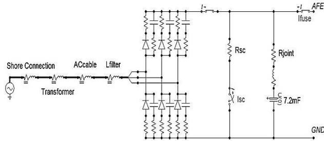
Fig. 4. ATP model of the shore connection converter in fault condition.
