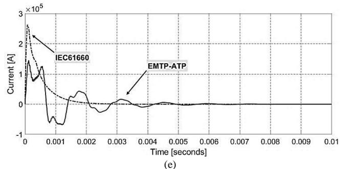
Fig. 6. Prospective short-circuit currents of ATP simulation (solid line) and IEC 61660-1 (dashed line). (a) Rectifier Converter. (b) Capacitor bank in the dc-link. (c) SWBD right-side from the fault point. (d) SWBD left-side from the fault point. (e) SWBD total contribution (fault current passing through 400 A high-speed fuse).
