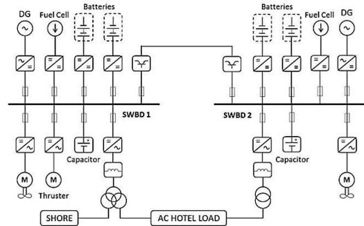
Fig. 2. ZEUS single line diagram (common dc bus topology).
