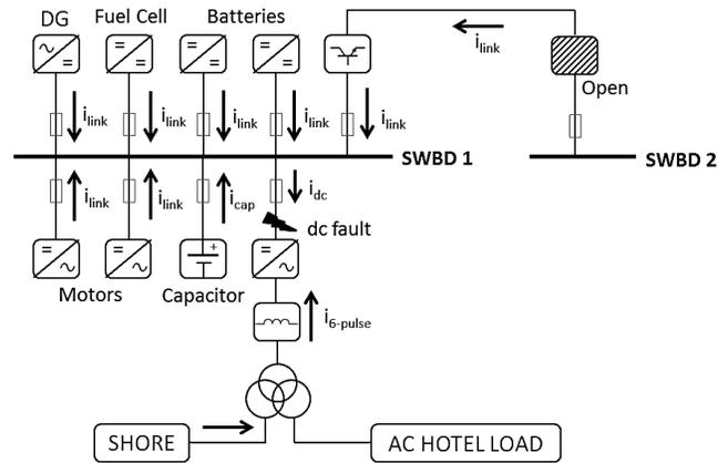
Fig. 5. Fault current flows on SOM Harbour.
