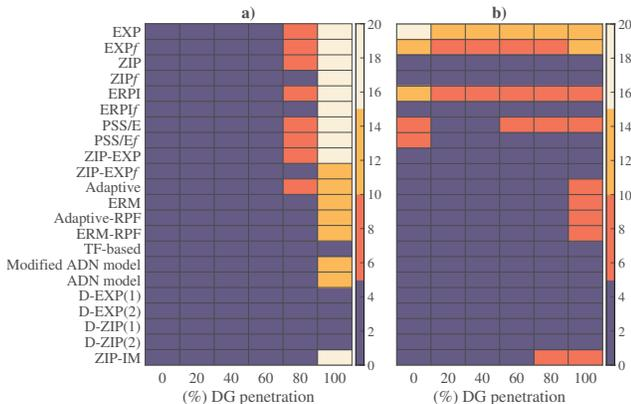
Fig. 4.  $\epsilon^t$  for a) real and b) reactive power as a function of DG penetration.
