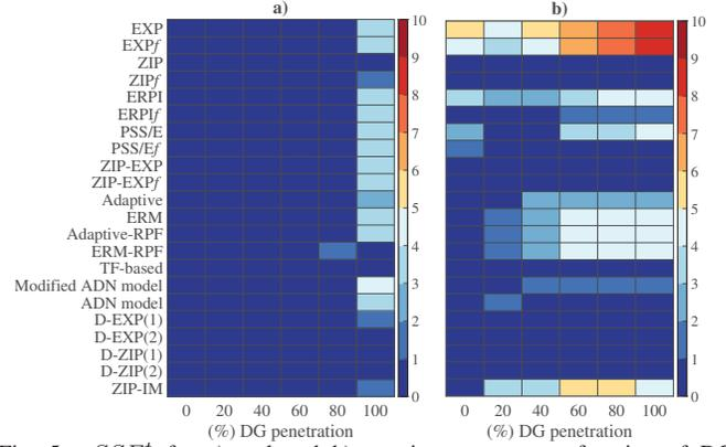
Fig. 5.  $SSE^t$  for a) real and b) reactive power as a function of DG penetration.
