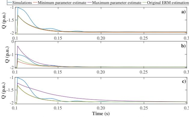
Fig. 7. Example for the proposed one-at-a-time sensitivity analysis using the ERM. Variation of a)  $N_s$ , b)  $N_t$ , and c)  $T_y$  parameters. The mathematical formulation and the description of ERM parameters are given in [9].
