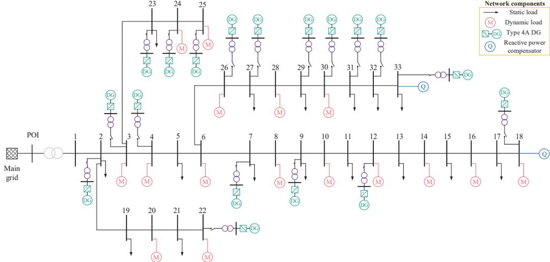
Fig. 2. Modified IEEE 33 bus distribution test system.
