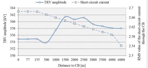
Fig. 9. TRV amplitude and short-circuit current to be interrupted at different fault distances from CB
