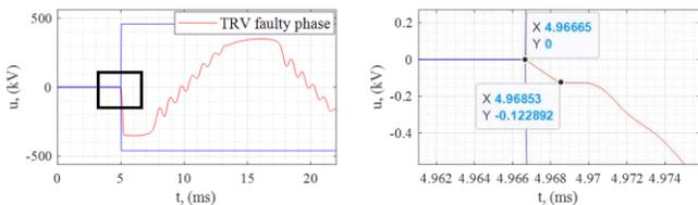
Fig. 8. TRV and the zoom of ITRV in case of SLF at the cable-OHL connection point
