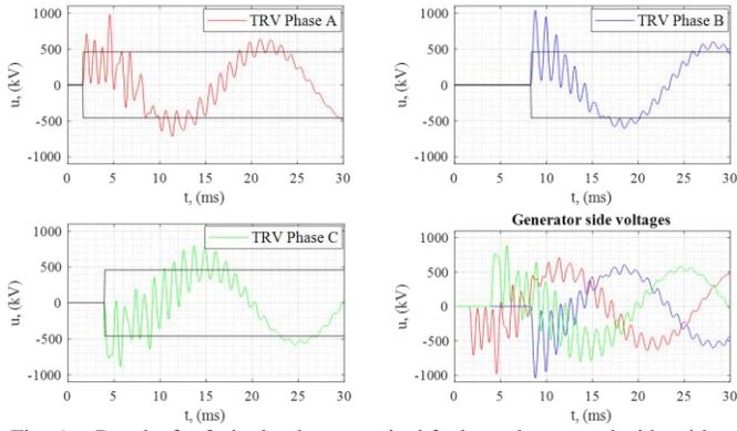
Fig. 6. Results for 3 single-phase terminal faults at the network side without surge arresters
