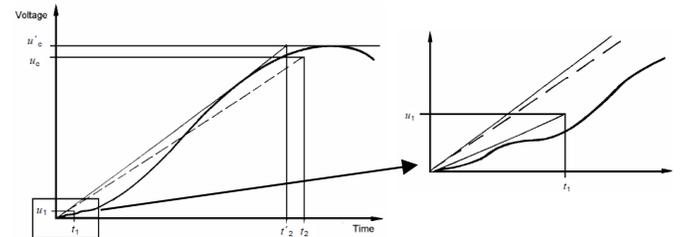
Fig. 10. TRV for capacitive current breaking tests, parameters  $u_c$ ,  $u_1$ ,  $t_1$  and  $t_2$  given in [2]
