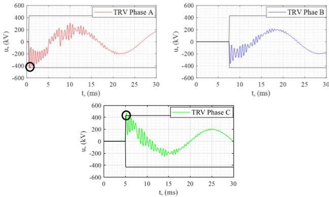
Fig. 7. Results for ungrounded three-phase fault on the generator side
