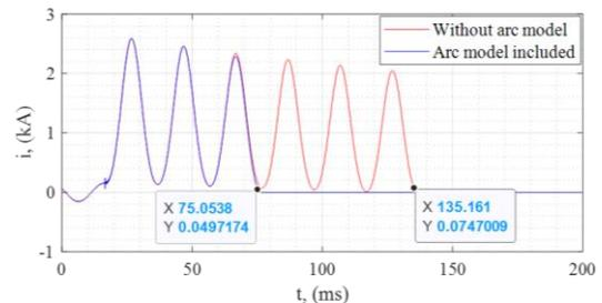
Fig. 12. Interrupting a short-circuit current in phase A. CB contact separation occurs at 60 ms. Current interrupted at 75 ms (arc included) and at 135 ms (without arc)
