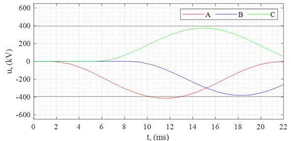
Fig. 11. TRV when breaking capacitive current of the unloaded OHL
