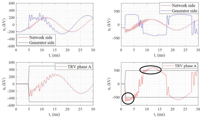
Fig. 3. Network and generator side voltages and TRVs when performing out-of-phase switching at angle 30° (left) and 180° (right)
