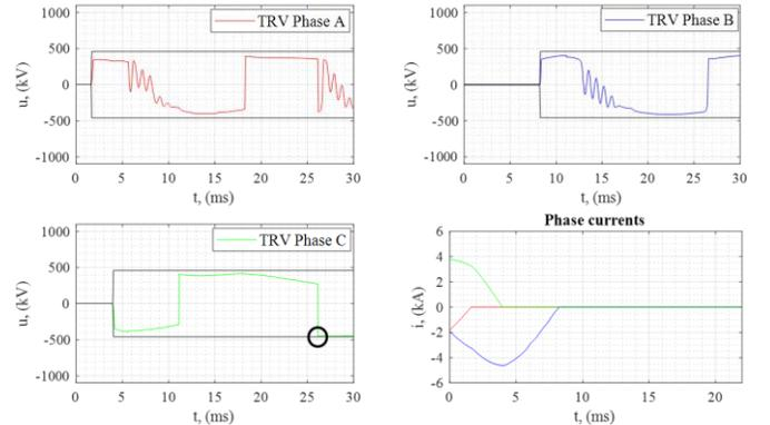
Fig. 4. Results for 3 single-phase terminal faults at the network side
