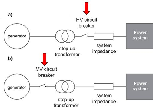
Fig. 1. Possible locations for circuit-breakers used for grid synchronizations 62271-37-013 [1] for generator circuit-breakers with rated voltages up to 38 kV, while IEC 62271-100 [2] covers requirements for high voltage circuit breakers.
