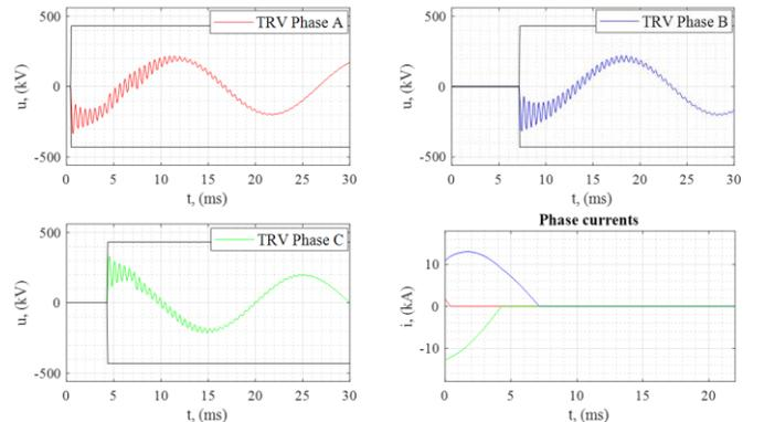
Fig. 5. Results for 3 single-phase terminal faults at the generator side
