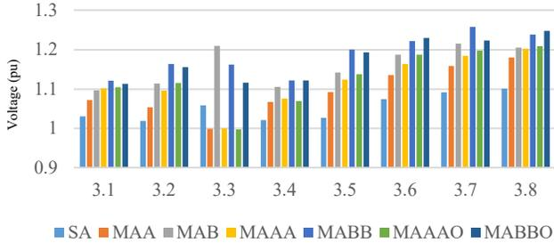
Fig. 9. Maximum onshore RMS voltages obtained in the fault cases for different topologies.
