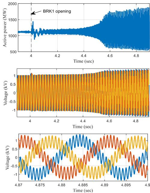
Fig. 13. Oscillations at the PCC of HVDC1 after opening of BRK1.
