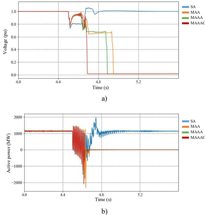
Fig. 7. RMS voltage (a) and active power (b) during phase-to-phase fault in different network configurations.
