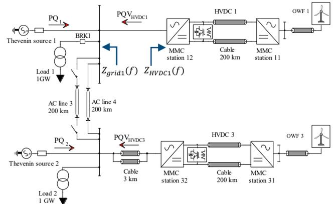
Fig. 12. Simulated network in the resonance study case.
