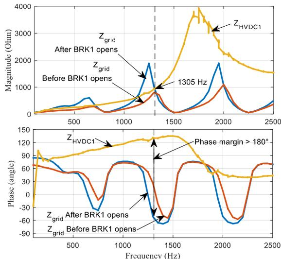
Fig. 14. Frequency response of HVDC1 converter station and grid impedance before and after opening of BRK1.
