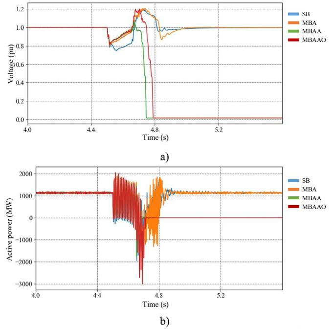
Fig. 8. RMS voltages (a) and active power (b) during phase-to-phase fault in different network configurations.
