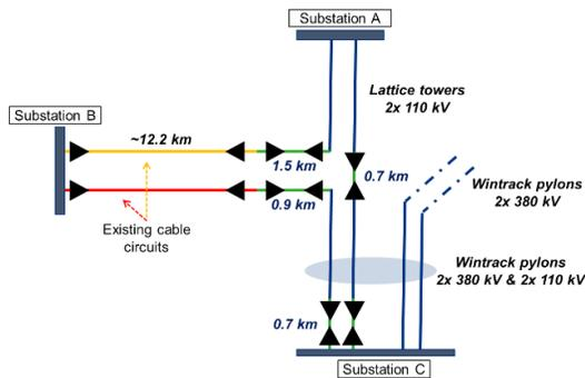
Fig. 1. Schematic of the 110 kV grid under study
