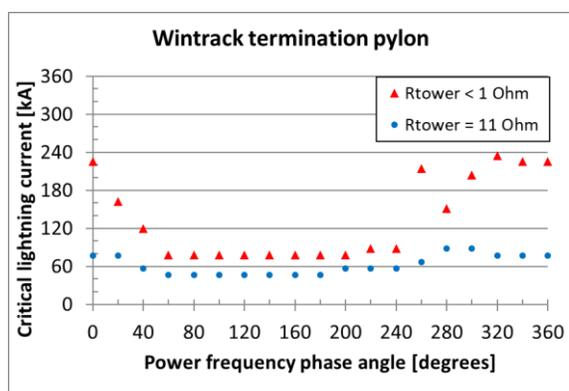
Fig. 10. Critical lightning currents for strikes on the Wintrack cable termination pylon
