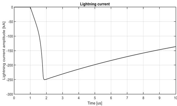
Fig. 7. Example of the applied lightning current waveshape in ATP
