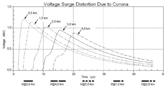
Fig. 4. Surge voltage waveforms at various distances from the strike location due to corona attenuation [5]
