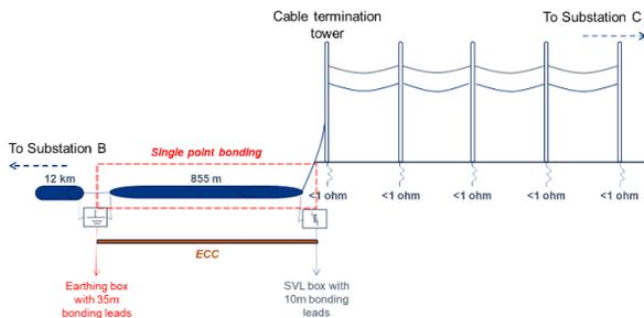
Fig. 3. Simplified schematic of cable circuit #2
