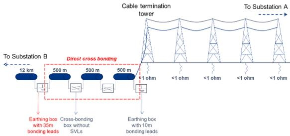
Fig. 2. Simplified schematic of cable circuit #1
