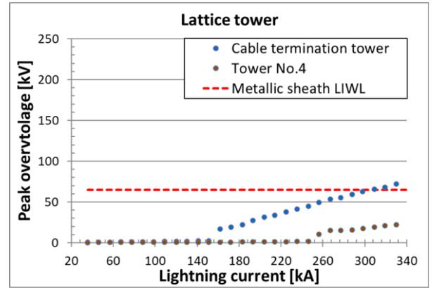
Fig. 8. Sheath peak overvoltages for lightning strikes on the lattice cable termination tower and on tower No.4
