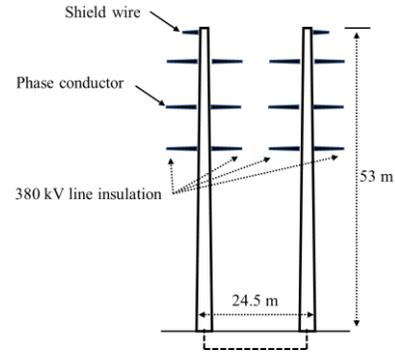
Fig. 6. Simplified schematic of the Wintrack pylons
