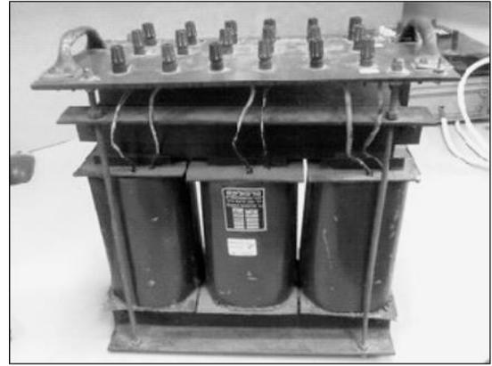
Fig. 2. 4.5 kVA dry type transformer
