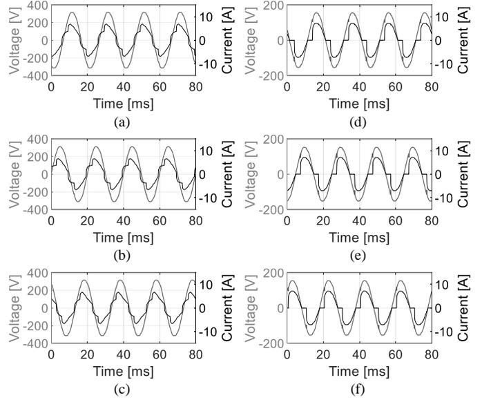
Fig. 5. Voltage and current waveforms for firing angle  $\alpha=45^\circ$ ; Primary side: (a) phase R, (b) phase S, and (c) phase T; Secondary side: (d) phase R, (e) phase S, and (f) phase T.
