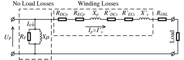
Fig. 1. Equivalent single-line transformer schematic.
