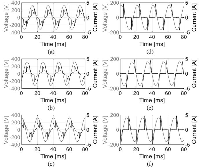
Fig. 6. Voltage and current waveforms for firing angle  $\alpha=135^\circ$ ; Primary side: (a) phase R, (b) phase S, and (c) phase T; Secondary side: (d) phase R, (e) phase S, and (f) phase T.
