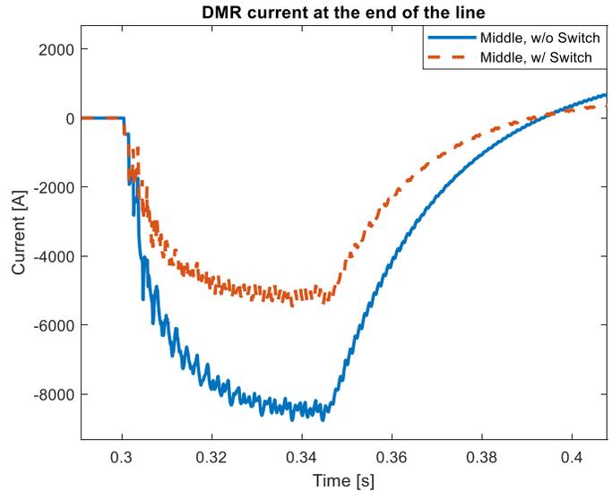
Figure 8 – The current of the DMR at the end of the line
