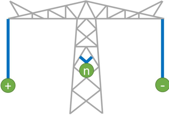
Figure 3 - HVDC overhead line tower and pole configuration
