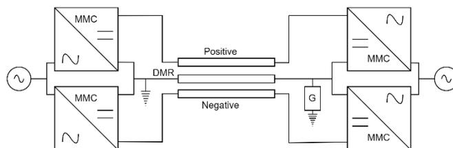
Figure 1 - HVDC bipolar system with DMR
