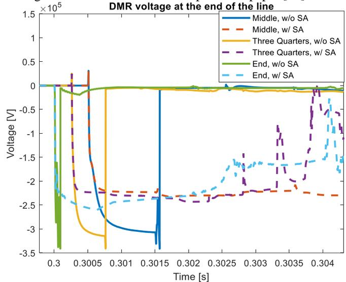
Figure 6 - DMR voltage measured at the end of the line for different fault locations
