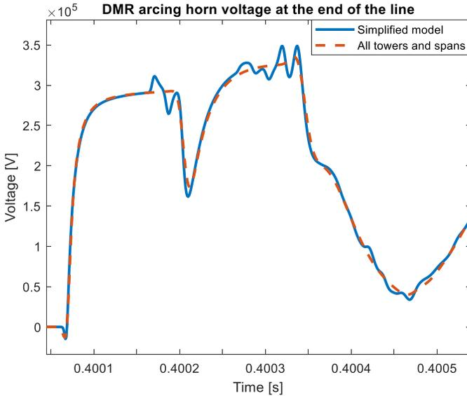
Figure 5 - DMR arcing horn voltage on a tower at the end of the line tower
