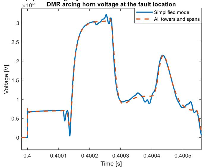
Figure 4 - DMR arcing horn voltage at the faulted tower
