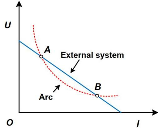
Figure 2 - U-I characteristic of an arc and the external system [5]
