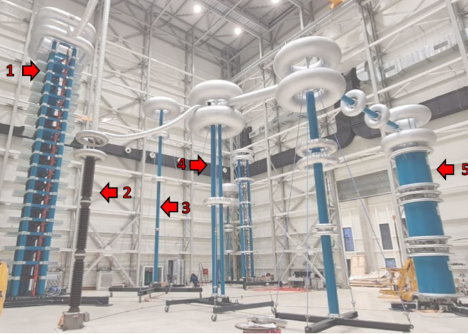
Fig. 1. Test setup in HV laboratory for superimposed impulse test (1 – impulse generator; 2 – test object (here a capacitor, but in observed case the DC cable test loop was used); 3 – impulse divider; 4 – universal divider; 5 – DC voltage generator)
