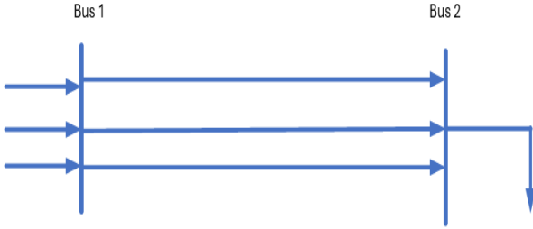
Fig. 3. Simple two bus system with unidirectional power flow to the load
