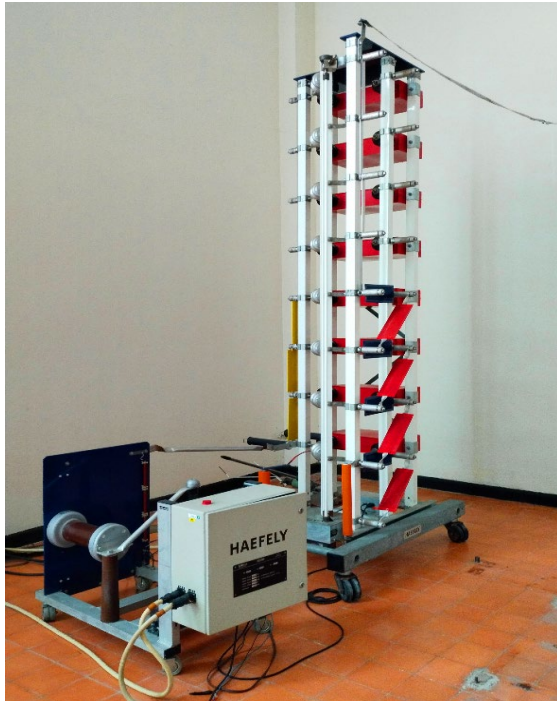
Fig. 3. The HAEFELY WO 533090 impulse generator used in the transformation ratio test.
