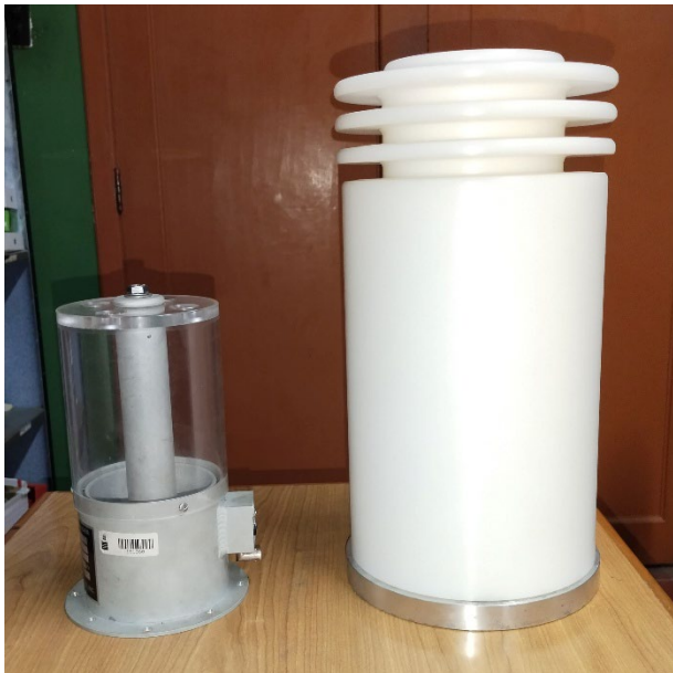
Fig. 1. Capacitive voltage divider: internal components (left) and their outer cover (right).
