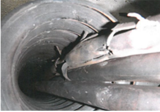
Fig. 18. Power cable damaged by lightning
