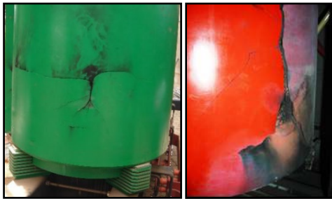
Fig. 3. Details of transformer failures during vacuum circuit breaker energization switching.
